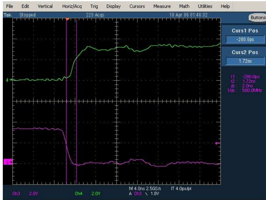
Figure 2.9: Measurements of a READY-WARN transition at the APVe FMM input connector. The purple trace represents the de-assertion of a READY state, whilst the green trace represents the assertion of a WARN state.
