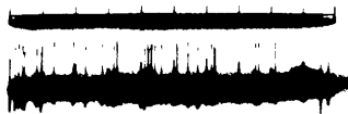
Fig. XXI-1. Unprocessed data played back from tape. Upper trace shows stimulus markers 1/sec (total time displayed, 10 sec). Large pulses on lower trace indicate firing of the neuron under study.
