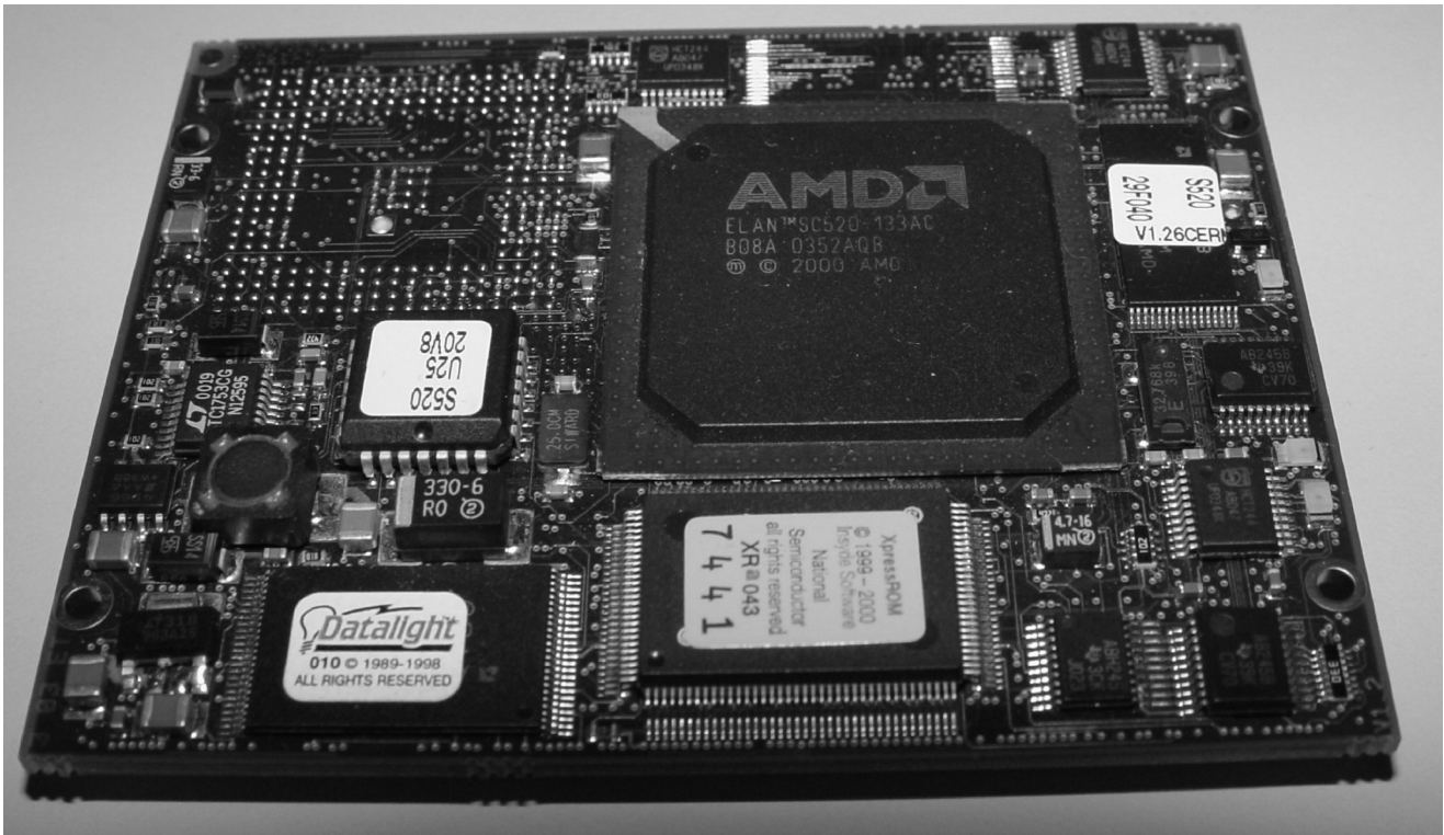
Fig. 1. Top-side of the SM520PCX embedded PC. The micro-controller together with some external components like the FLASH-RAM for the BIOS can be seen. A standard SO-DIMM memory-module, normally used in portable computers, is on the back.
