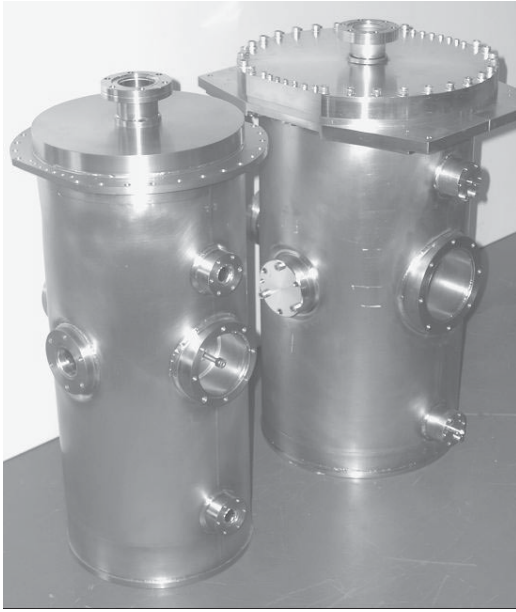
FIG. 1. The INFN-LNL low- \beta (left) and medium- \beta 352 MHz superconducting half-wave resonators.
