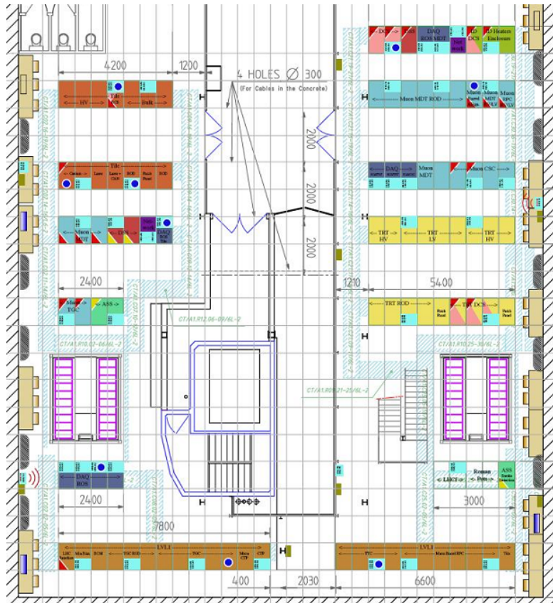
Figure 2.4: Electronics racks distribution in the underground USA15 level 1. Different sub-detectors' racks (represented by colors) that will allocate the instrumentation, mainly rack mounted PCs and the power systems. [14].
