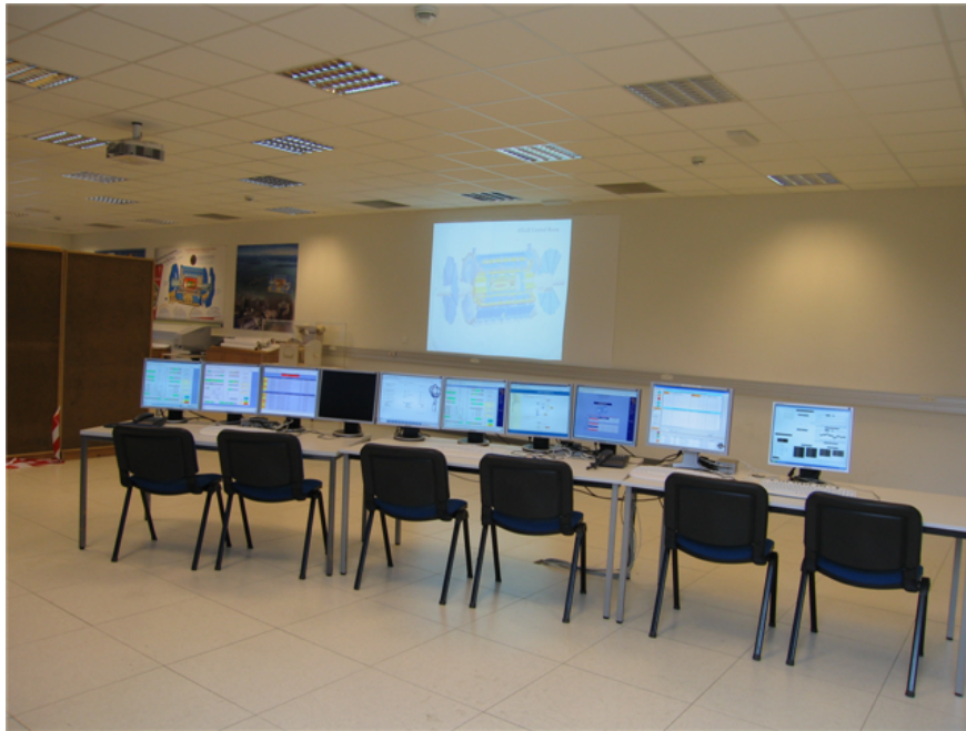
Figure C.2: Prototype of ACR in operation since April 2006. Various screens where the DCS top level interface is running. At that time however, the control was 'taken' from underground, where much of the work was being carried out.
