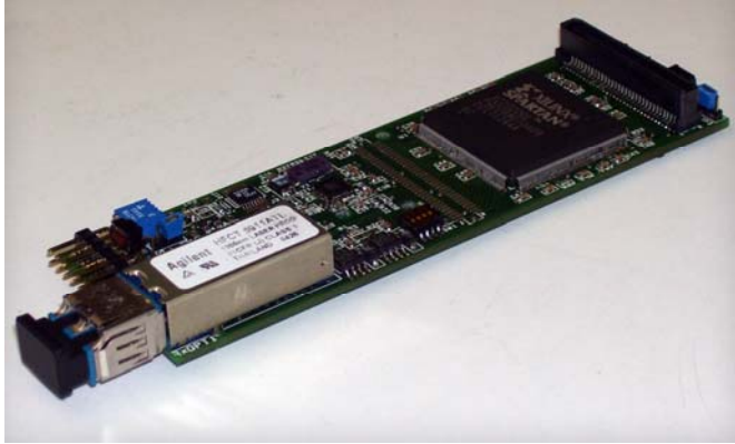
Figure 3: The trigger emulator plug-in module. On the left, the optical transceiver is shown while on the right, the FPGA and the mezzanine connector.
