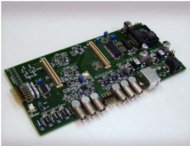
Figure 4: Photograph of the support board that provides power, additional clock, JTAG and USB interface to the trigger emulator mezzanine, used for evaluation purposes.
