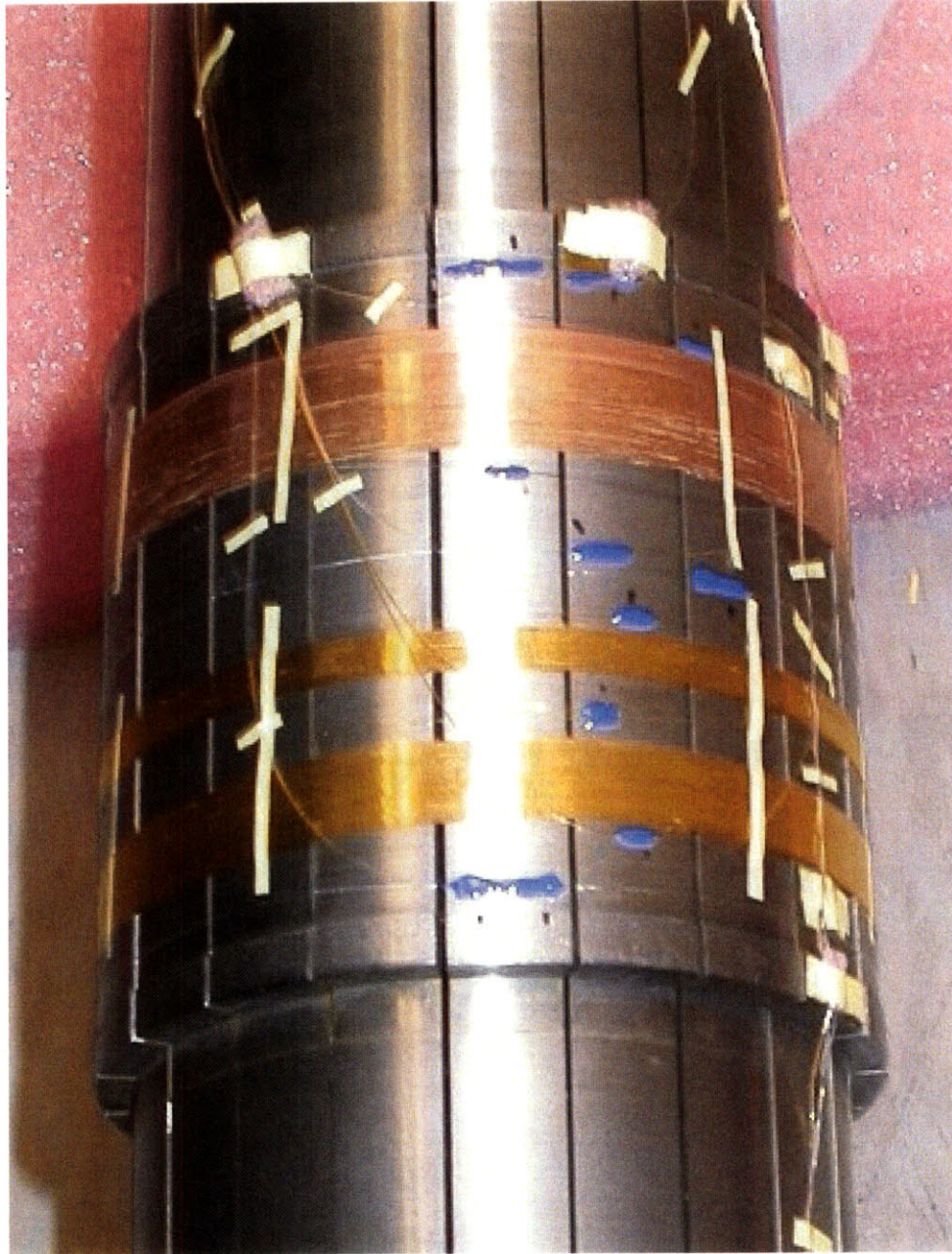
Figure 4-21: Final view of the strain probe.
