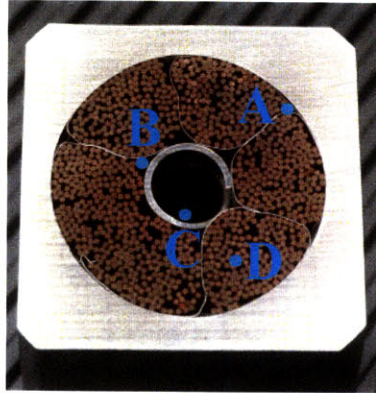
Figure 2-15: The fiber can be placed in the valleys due to the winding, in the central cooling channel, or co-wound with the superconducting wires.
