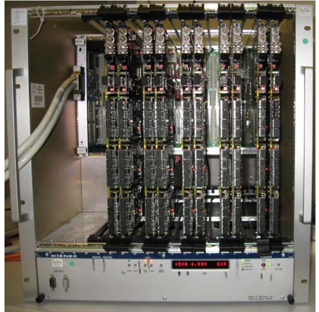
Figure 8: 9U/6U VME crate with 10 final SPD Routers
