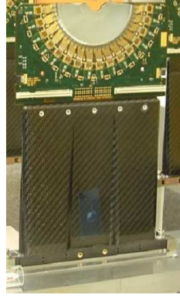
Figure 3: A VeLo module. The main components shown are the paddle, the hybrid, the front end chips and the sensor.
