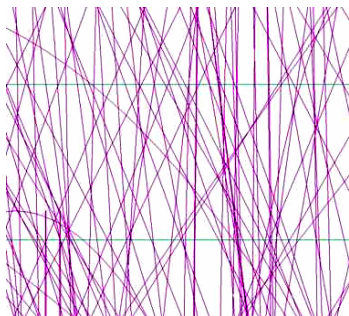
Figure 1: Track overlap in y-z plane (detector coordinates – see Fig. 3). 1cm layer separation is denoted by the two cyan lines. Note the significant overlap of tracks between these two layers, which will hinder tracker reconstruction.
