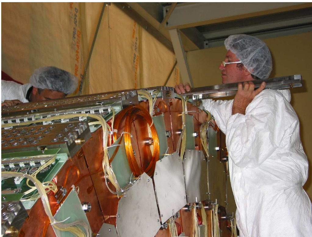
Figure 14. A view showing technicians assembling the wheel alignment key prior to wheel insertion into the cryostat.
