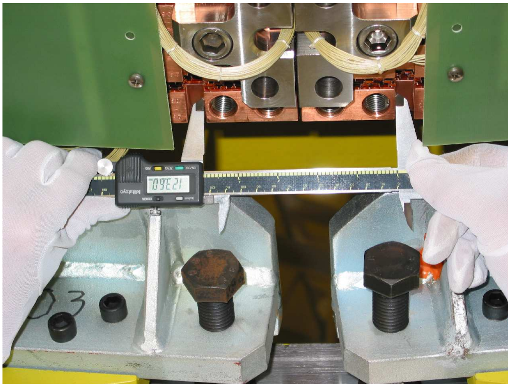
Figure 12. Final adjustment of module-to-module spacing, prior to installing the connection bars on the outer diameter of the detector wheel.
