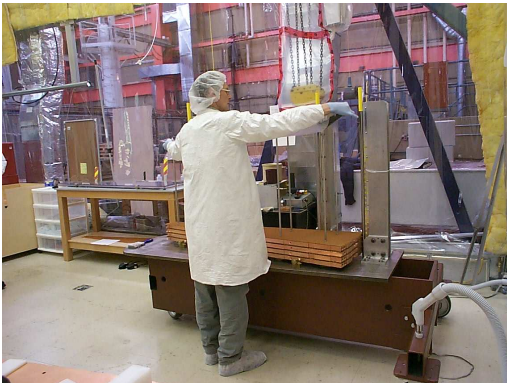
Figure 8. Stacking table with a partly stacked module. The module assembler is shown carefully lowering a EST board onto the 7 vertical stainless steel tie rods. When completed this front module will consist of 25 copper plates, with 24 8.5 mm gaps filled with the honeycomb/electrode structure.
