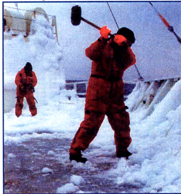
Figure 6.1: Deck Ice Removal
