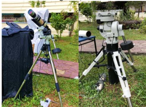
Figure 2. Borg 76 mm refractor mounted on CEM25P mount (left) and CEM60 mount (right)
