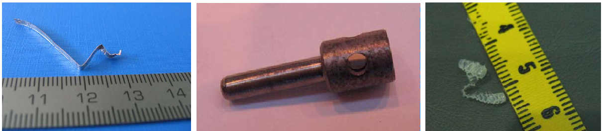
Figure 1. Some of the objects found along the beam pipe in the LHC magnets [3].
