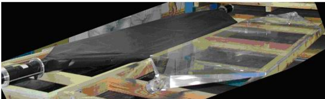
Fig. 14 Picture of scintillator slabs with their lightguides. One of them is already wrapped with black plastic sheet and two phototubes are seen as well.
