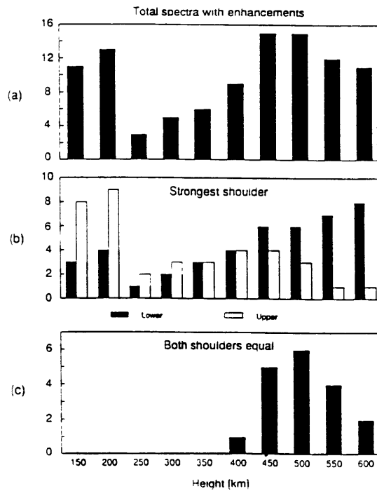
Figure 6-4: Histograms showing the height distribution of enhanced ion acoustic spectra categorized by a) total enhanced spectra; b) upshifted or downshifted peak enhancement; and c) both peaks enhanced symmetrically [after RD91].
