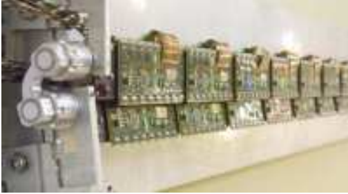
Fig. 6. View of a bistave, two barrel staves connected by the same cooling line.
