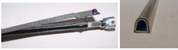
Fig. 8. Example of a delaminated stave (left). The pipe insertion solution to the leak problem (right).
