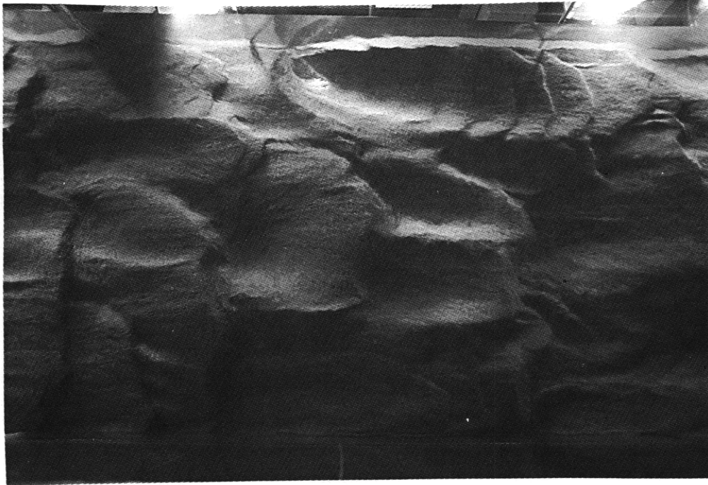
Figure 5-10. Plan view of sediment bed. (Run 9-5, V = 47.4 , centered at 850 cm, length of field of view = 155 cm, flow from left to right)
