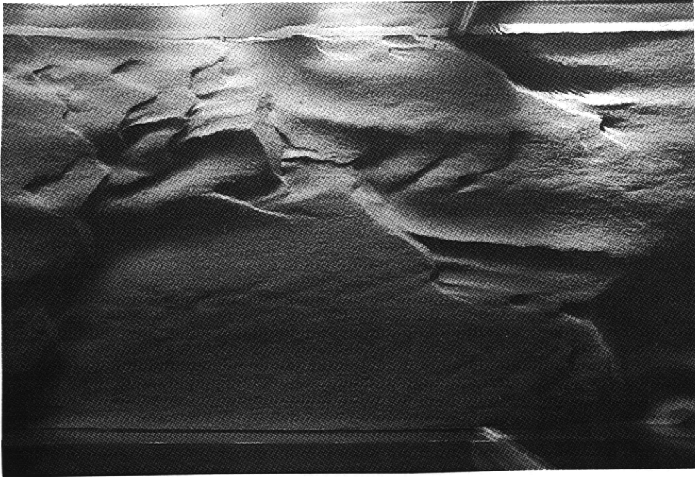
Figure 5-12. Plan view of sediment bed. (Run 11-2, V = 38.4 cm/s, centered at 750 cm, length of field of view = 155 cm, flow from left to right)
