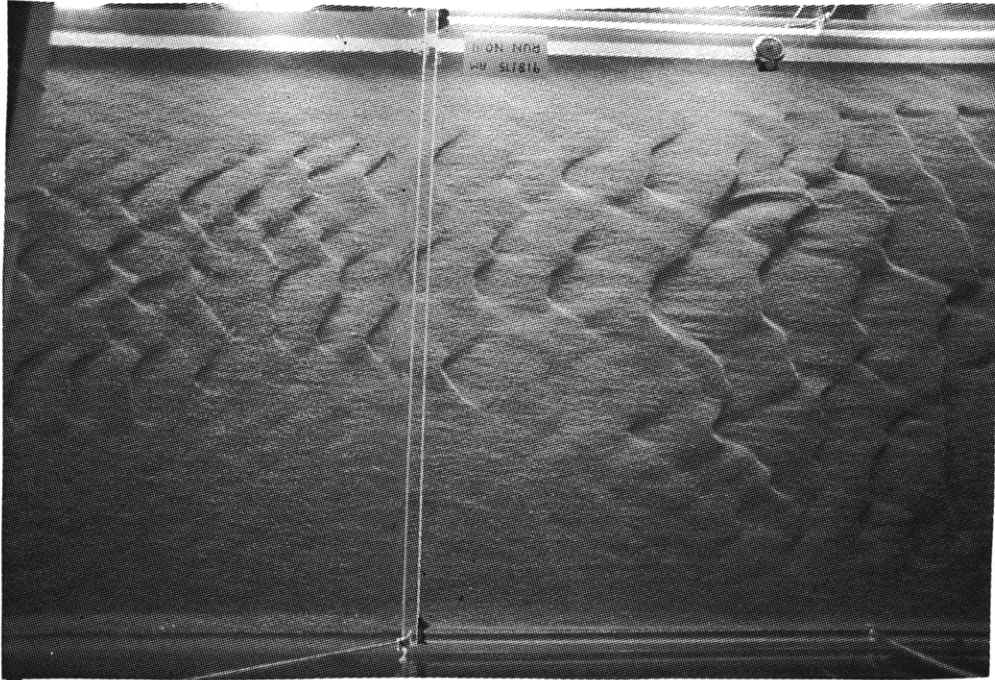
Figure 4-29. Plan view of sediment bed underneath the water-surface plate and immediately upstream from the plate 12 minutes after start-up (overlaps with Figure 4-30). (Run 11-1, V = 38.4 cm/s, centered at 650 cm, length of field of view = 155 cm, flow from left to right)
