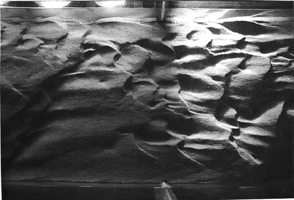
Figure 5-13. Plan view of the same section of the sediment bed as in Figure 5-12, one hour and 35 minutes after Figure 5-12 was taken. Figures 5-12 and 5-13 illustrate relatively long bed forms being broken up by the development of smaller bed forms on their stoss side. See text. (Run 11-2, V = 38.4 cm/s, centered at 770 cm, length of field of view = 155 cm, flow from left to right)
