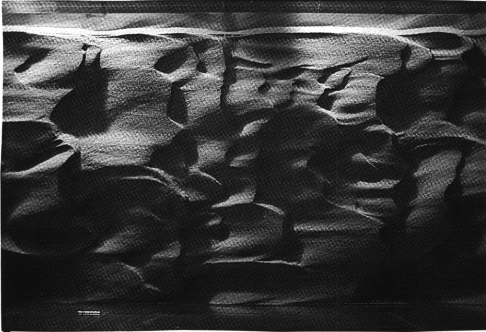
Figure 5-14. Plan view of sediment bed. (Run 10-3, V = 32.3 cm/s, centered at 880 cm, length of field of view = 155 cm, flow from left to right)
