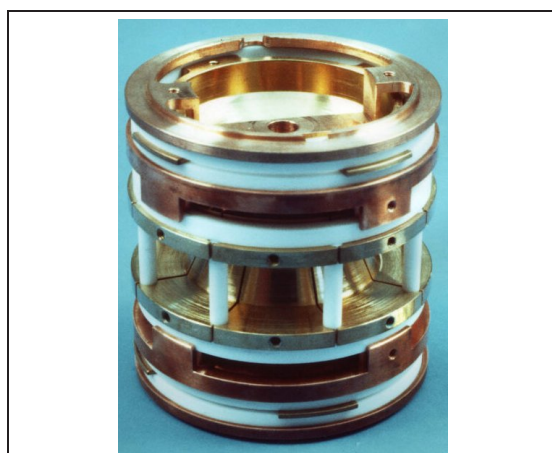
FIGURE 4.8: Photo of the hyperbolic Penning trap of ISOLTRAP 1 .
