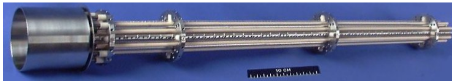
FIGURE 4.4: Photo of the radio frequency quadrupole (RFQ) of ISOLTRAP [Herf01b].
