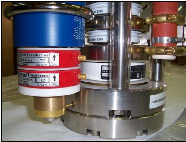
Fig. 2. Re-trigger CTs in the main discharge switch.
