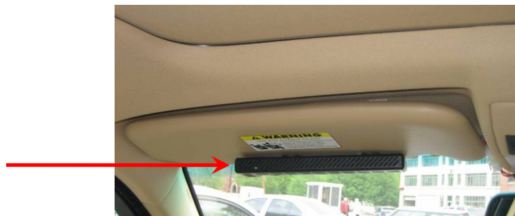
Figure 3: Array microphone used to detect user's voice
