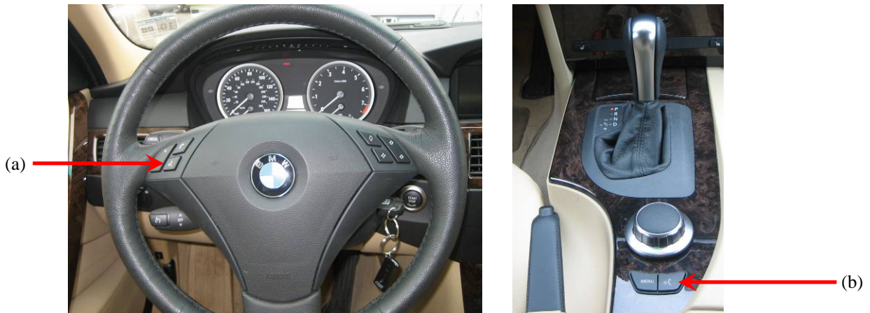
Figure 2: Speech buttons (a) steering wheel speech button; (b) iDrive speech button
