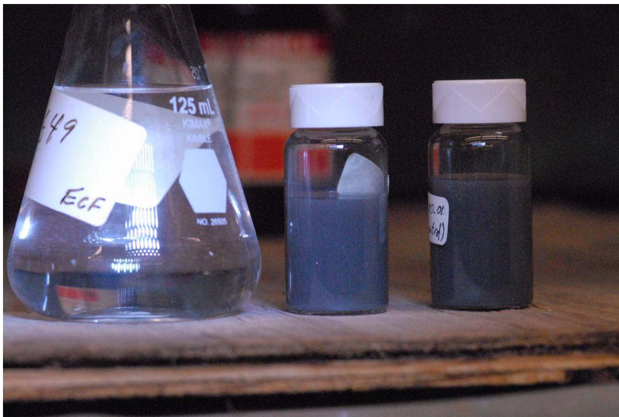
Figure 42: (Left) Pure Novec 649; (Middle) 0.01vol% Aluminum in Novec 649 with Fluorinated Surfactant ~1 hour after preparation; and (Right) 0.01vol% Aluminum in Novec 649 w/o surfactant ~40 minutes after preparation. Note that both samples appear relatively well-dispersed.
