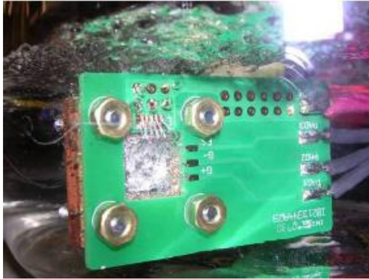
Figure 40: Dual Side Immersion Cooling of an IGBT Die Soldered to a Copper Boiler in a Hydrofluoroether Working Fluid. Reproduced with permission of Phil Tuma, 3M Electronics Markets Materials Division, 2008.
