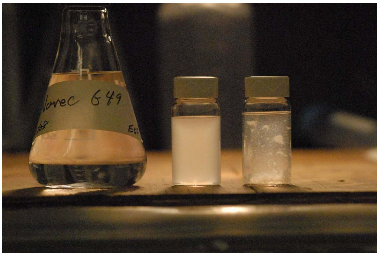
Figure 41: (Left) Pure Novec 649; (Middle) 0.01vol% SiO 2 in Novec 649 with Fluorinated Surfactant ~1 hour after preparation (Middle); and (Right) 0.01vol% in Novec 649 w/o surfactant ~40 minutes after preparation. Note that the sample without the surfactant is heavily flocculated, whereas the sample with surfactant appears well-dispersed.
