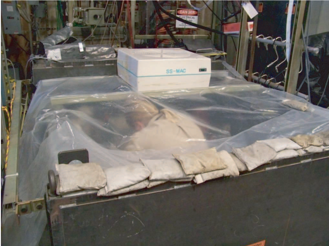
Figure 6-11: Photograph of PBG structure being installed in lead enclosure for breakdown testing.
