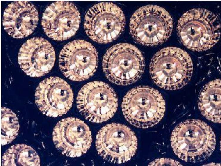
Figure 3-2: A view of the SNO photomultiplier tubes. Note the flower petal-like reflectors around each PMT. These serve to increase the photocathode coverage of the detector by 75%.
