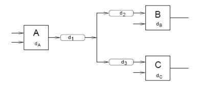
Figure 2-10: A circuit fragment with gate and wire delays for illustration of different asynchronous circuit classes, courtesy of [64].
