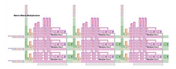
Figure 2-7: An ALA schematic implementing multiplication between two  $3 \times 3$  matrices, each element of the matrices is a 3-bit number, courtesy of [24].
