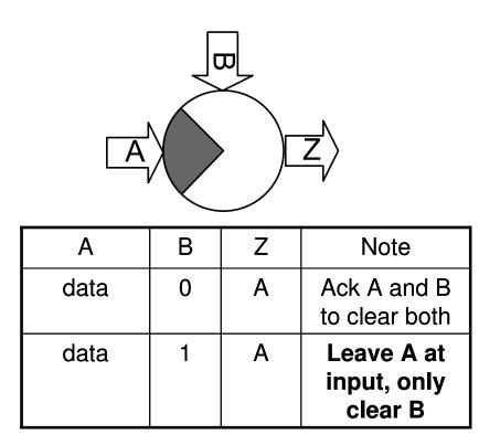
Figure 3-11: The COPY cell definition.
