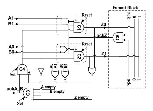
Figure 3-4: Block level design of the NAND cell in the ALA cell library.
