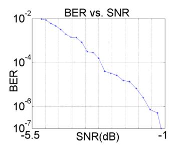
Figure 6-5: 7-bit NLL test results: the Bit Error Rate vs. the Signal-to-Noise Ratio plot.
