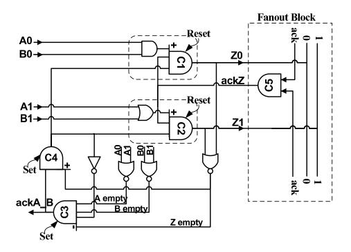
Figure 3-5: Block level design of the OR cell in the ALA cell library.
