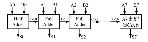
Figure 4-1: The block diagram of the 8-bit ripple adder.
