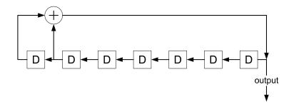
Figure 6-1: 7-bit LFSR transmitter.
