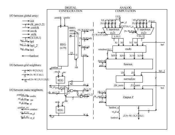
Figure 5-5: Block diagram of one AnLA cell.
