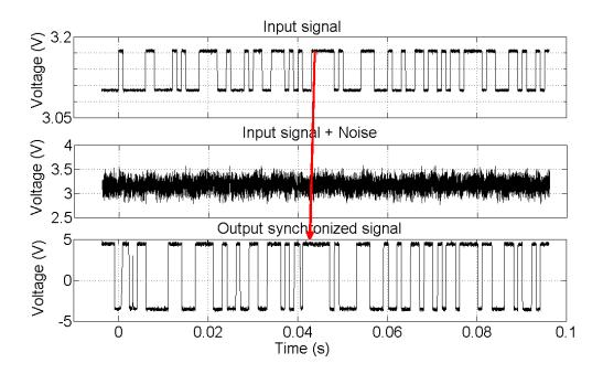
Figure 6-4: 7-bit NLL test results: the locking and tracking dynamics.
