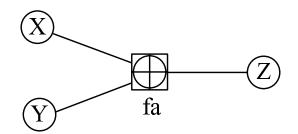
Figure 5-2: Factor graph representation of a soft XOR gate.
