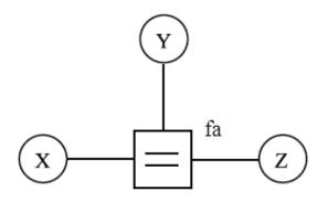
Figure 5-3: Factor graph representation of a soft EQ gate.
