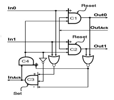
Figure 2-17: The schematic of a PCFB, courtesy of [80].
