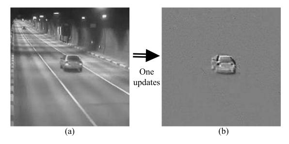
Figure 6-10: Motion detection effect after AnLA processing: (a) One frame from a traffic video; (b) Motion detection effect.
