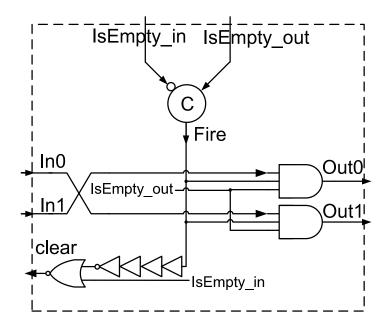
Figure 3-21: The implementation of the cell interface with an INV function embedded.
