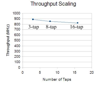
Figure 4-9: Throughput vs. number of taps in the FIR filter.
