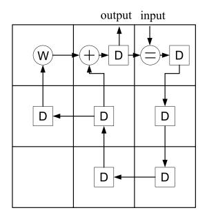
Figure 6-3: 7-bit NLL receiver implemented on  $3 \times 3$  AnLA.
