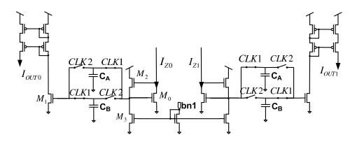
Figure 5-8: Analog storage and output stage.
