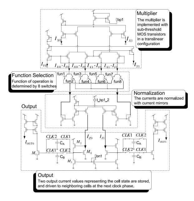
Figure 5-9: Core schematic of an AnLA cell.
