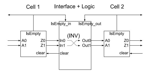
Figure 3-19: A block diagram showing self-timed asynchronous cells and the interface: tokens are inverted by the asynchronous interface and propagated from Cell 1 to Cell 2 in this example.
