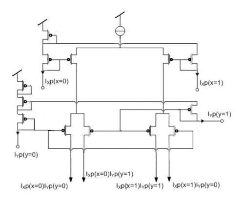
Figure 5-6: Schematic of a Gilbert Multiplier.
