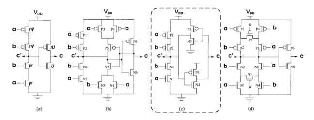
Figure 3-14: Different CMOS implementations of the C-element, courtesy of [59].
