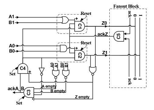
Figure 3-6: Block level design of the NOR cell in the ALA cell library.
