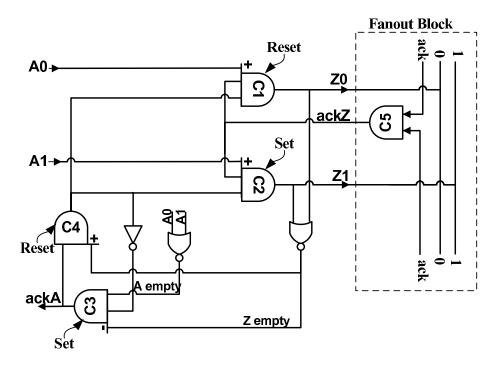
Figure 3-8: Block level design of the BUF cell initialized to "T" (BUF\_T) in the ALA cell library.
