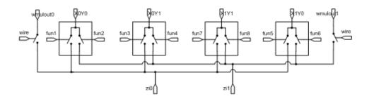
Figure 5-7: Switching function mux.
