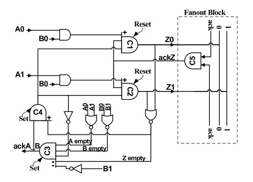
Figure 3-12: Block level design of the DELETE cell in the ALA cell library.
