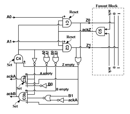
Figure 3-13: Block level design of the COPY cell in the ALA cell library.
