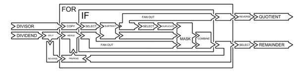
Figure 2-6: A integer divider schematic implemented on ALA, courtesy of [24].
