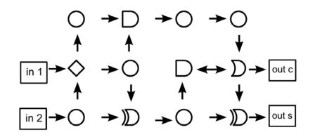
Figure 2-3: A serial adder schematic implemented on ALA, courtesy of [24].
