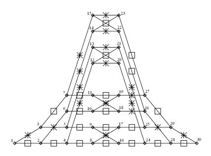
Figure 6-6: The trellis of the (7, 4) Hamming code.
