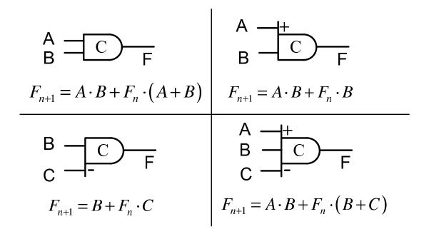
Figure 2-15: Variants of C-element, symbols and equations.
