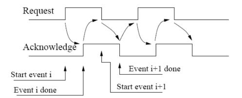
Figure 2-12: The two-phase handshake protocol, courtesy of [11].
