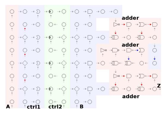
Figure 4-12: Serial 4-bit multiplier implemented in ALA.
