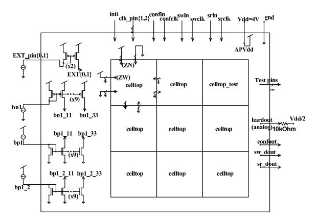
Figure 5-4: Architecture of a  $3 \times 3$  AnLA array.
