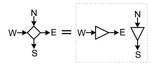
Figure 3-9: Block level design of the CROSSOVER cell in the ALA cell library.
