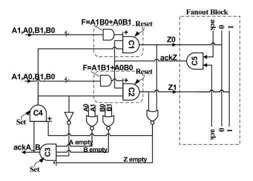
Figure 3-7: Block level design of the XOR cell in the ALA cell library.
