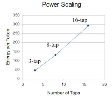
Figure 4-10: Energy consumption vs. number of taps in the FIR filter.
