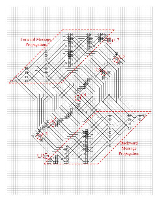
Figure 6-7: AnLA array schematic for (7, 4) Hamming code decoding.
