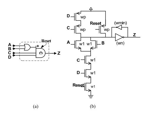
Figure 3-15: An C-element with multiple, asymmetric inputs and OR function: (a)the block level symbol; (b) the CMOS implementation.
