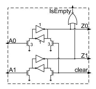
Figure 3-20: The implementation of the cell state storage for self-timed ALA.
