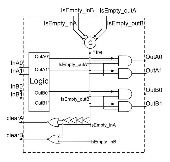
Figure 3-22: The implementation of the cell interface for general functions, two inputs and two outputs.
