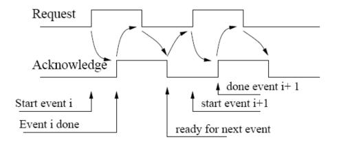
Figure 2-11: The four-phase handshake protocol, courtesy of [11].
