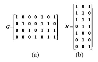
Figure A-1: Matrix representation of a (7, 4) Hamming code: (a)the generator matrix G; (b) the parity-check matrix H.
