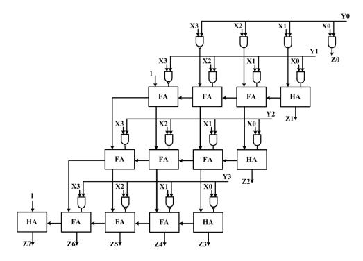
Figure 4-4: The block diagram of a 4-bit signed multiplier.
