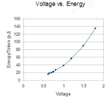
Figure 4-7: Power supply voltage scaling effect on the energy consumption of the FIR filter.
