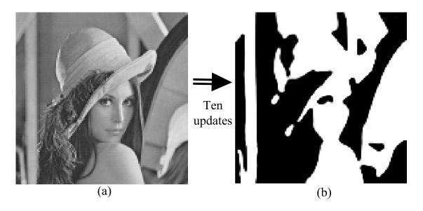
Figure 6-8: Segmentation effect after AnLA processing: (a) Original image; (b) Segmented image after 10 updates.
