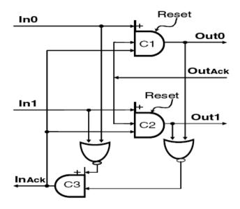
Figure 2-16: The schematic of a PCHB, courtesy of [80].
