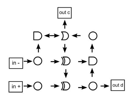
Figure 2-4: A subtracter schematic implemented on ALA, courtesy of [24].
