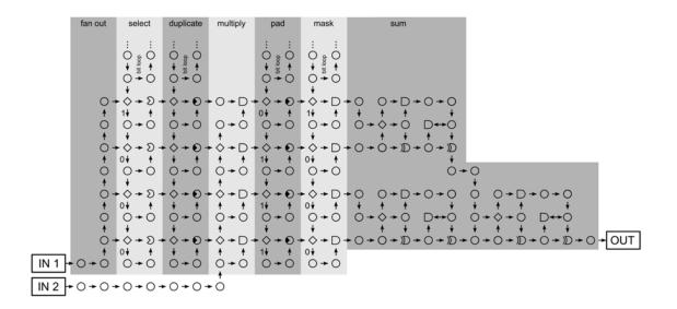
Figure 2-5: A multiplying schematic implemented on ALA, courtesy of [24].
