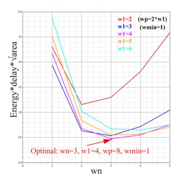
Figure 3-16: Circuit sweep simulation showing the transistor sizing optimum.
