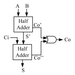
Figure 4-3: The logic diagram of a full adder.
