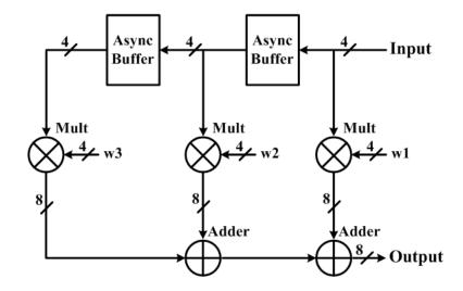
Figure 4-5: The block diagram of a 4-bit 3-tap FIR filter.
