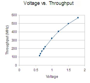
Figure 4-6: Power supply voltage scaling effect on the throughput of the FIR filter.
