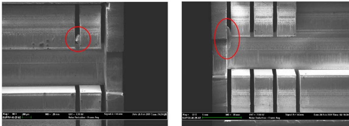
Figure 6-8: SEMs showing shorting from stringers
