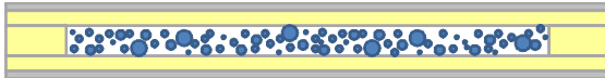
Figure 1. Blast mitigation composite structure material sample: Plexiglass (gray), VN-600 foam (yellow), filler (blue).
