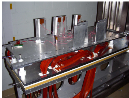
Figure 36: Cooling plate equipped with 8 balconies carrying Kapton heaters, which were serially connected to a power supply.
