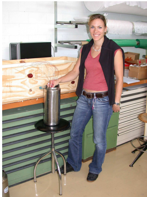
Figure 27: Calibration of PT1000 sensors in ice water.
