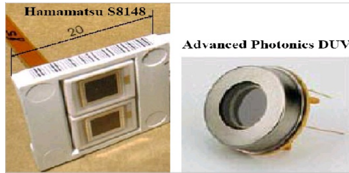
Figure 8: Two types of APDs used in the beam test.
