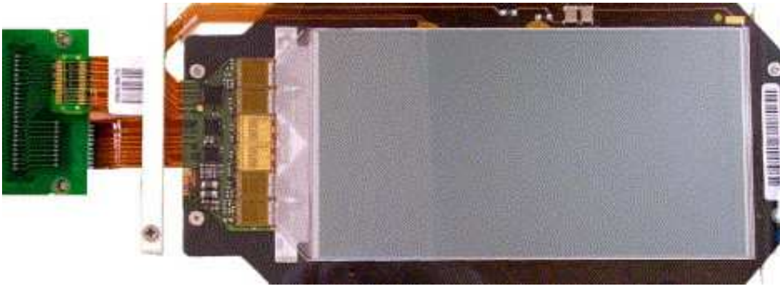
Figure 3: A module for the CMS tracker inner barrel (TIB). The external black structure is the carbon fiber frame. The larger rectangular central grey area is the silicon sensor, surrounded by the kapton circuit for insulation and bias. At the left edge of the sensor, in light grey, is the glass pitch adapter, bringing the signal to the front-end hybrid and chips, on the far left of the frame, and to the cable out of the module on the left.
