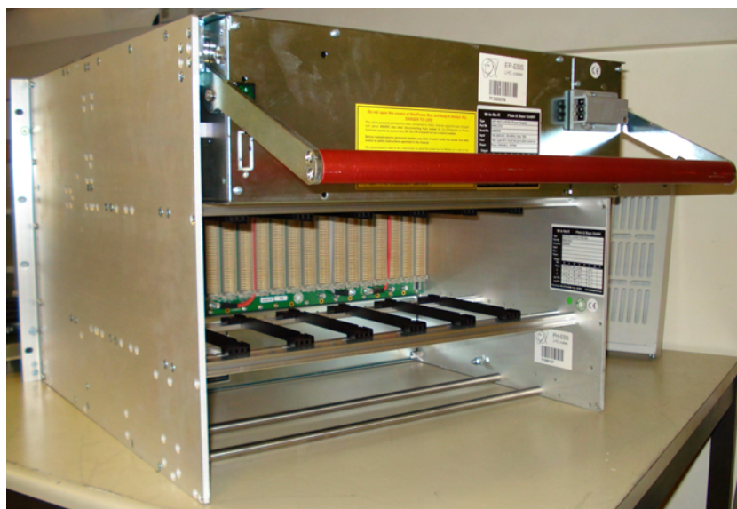
Figure O.1: Rear of an Empty VME Chassis Equipped with a Card Cage
