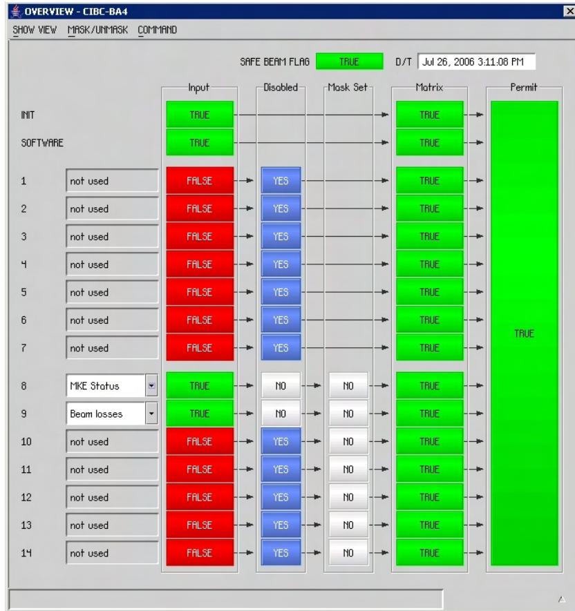
Figure 5.17: Controller Supervision Screen Prototype, SPS 2006
