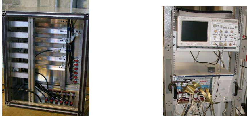
Figure 9: Electrical tests setup: the light-proof box (left) and the readout boards installed in the VME crate (right).
