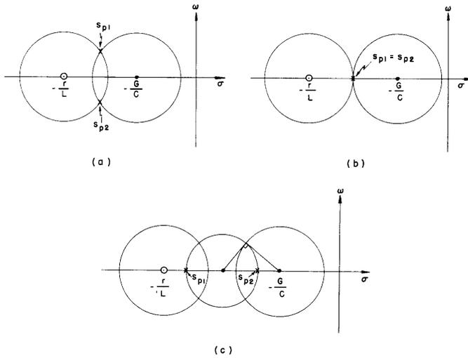
Fig. XIII-1. Graphical construction of pole positions.
