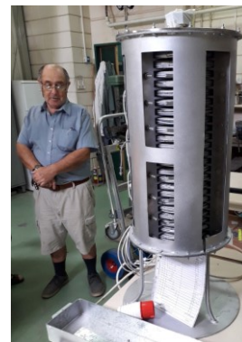
Fig. 7. A picture of the high temperature ( 300^{\circ}\text{C} ) liquid Lithium ALIN pump
