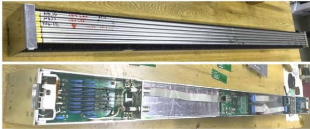
**Fig. 1.** PSD system of 1 m length and 8 mm diameter.
