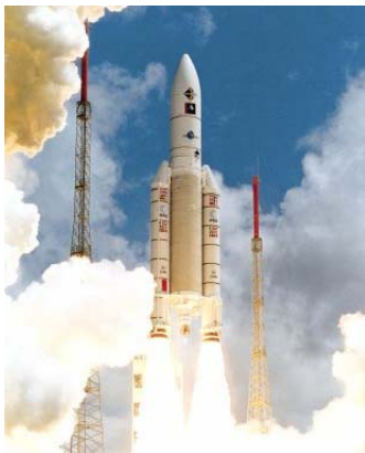
a) Ariane 5 (25 t liquid hydrogen, 130 t liquid oxygen)
