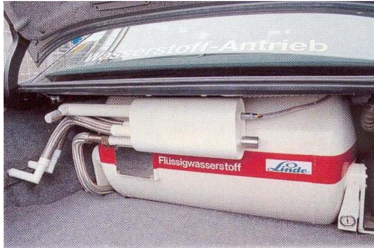
Figure 4 Automotive liquid hydrogen fuel tank
