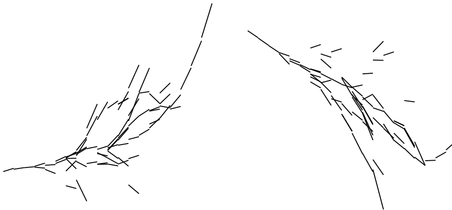
Figure 2. xz projection (left) and yz projection (right) of a reconstructed shower generated by a 6 GeV electron interacting in the \sim 3.3 X_0 ECC exposed at DESY. Each segment corresponds to a base-track associated with the reconstructed electromagnetic shower.
