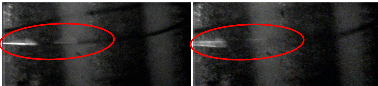
Figure 1. Photographs of a wire-bonds: left) off resonance; right) on resonance (17kHz).
