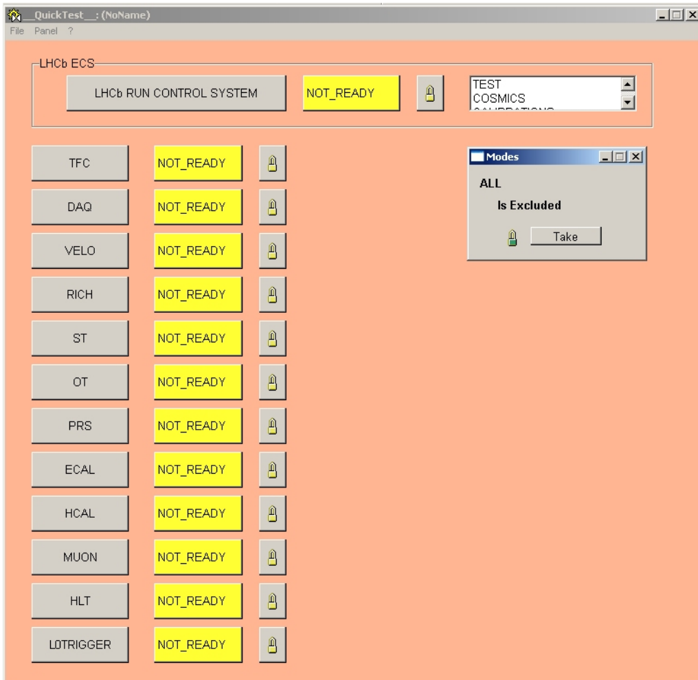
Figure 28. Very simplified LHCb RUN CONTROL PVSS panel.
