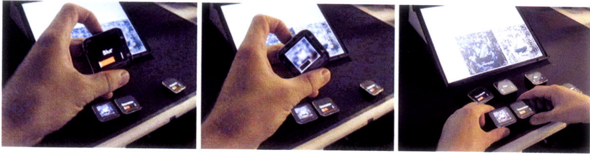
Figure 6-6: The Siftables version of the image manipulation application. On the left, a participant has lifted the Blur Siftable off the table, and tilted it to the left to adjust the value. In the center, the value is being adjusted as a result of the tilt (note that the on-screen visuals have changed to an effect preview). On the right the participant is applying an effect to the image by placing the effect Siftable to the right of the image Siftable, inserting it into the active effect chain.
