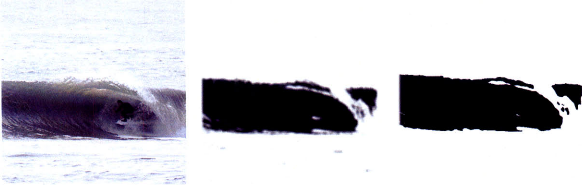
Figure 6-4: An original image (left), the original image with effects Threshold then Blur applied (middle), and the original image with effects Blur then Threshold applied (right). The order of the effects makes a difference to the end result.
