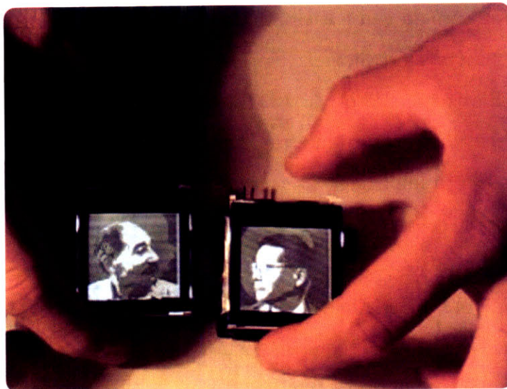
Figure 3-9: The “Attentionables” application was programmed for the Second Electronic Prototype by Evan Broder. Siftables detect each other using infrared when placed side-by-side, and each face looks towards the other. Attentionables adapts an art piece by Zuckerman and Sadi, and it was the first real application that extended Siftables’ behavior beyond the level of a simple application sketch.
