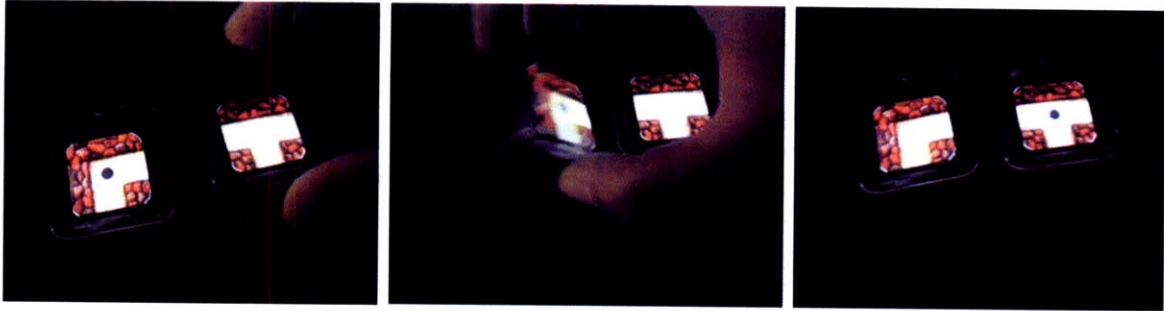
Figure 4-7: A maze exploration game illustrates some methods for navigating structures that are too large to be completely represented on the screen of a collection of Siftables at a single instant. The user can “dump” their character from one position to an adjacent position and can view a summary of the already-explored territory.
