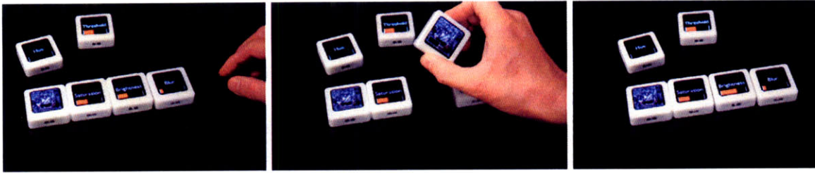
Figure 4-14: Image Manipulation application: Adjusting the brightness parameter by lifting and tilting the “brightness” Siftable, the placing it back into the filter chain. While the adjustment is in progress, the Siftable’s screen shows a live preview of the effect, then once it is placed down again it reverts to showing the name of the effect and red value-bar.
