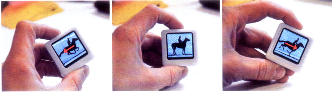
Figure 4-18: The tilt-to-roll video sketch utilizes Muybridge’s classic series of photographs titled “The Horse In Motion.” When the user tilts the Siftable to the right (right image), the frames advance in the forward direction and a right-pointing red arrow is superimposed. When tilted to the left (left image), they proceed in reverse with a left-pointing arrow. When the Siftable is flat (center image), the “at rest” image is displayed.
