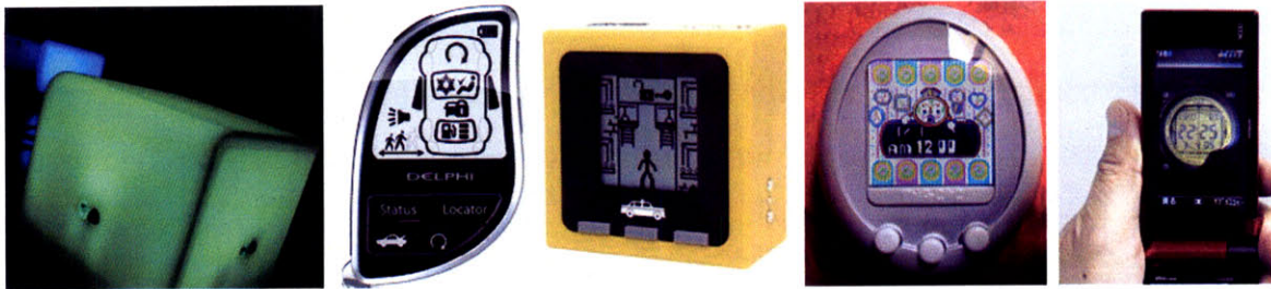
Figure 3-5: A subset of different display possibilities that were considered for Siftables. From left to right, they are single-color (essentially 1 pixel of information), black and white segmented, black and white bitmap, color bitmap, and three-dimensional. Depicted products are (from left to right) AudioCubes [95], Delphi key fob [21], Cube World [33], Tamagotchi [7], and the Hitachi Wooo H001 mobile phone [24].
