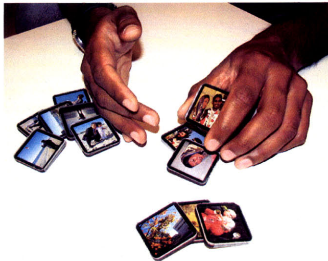
Figure 3-6: Paper, wood and acrylic mockups. The given size and thickness were selected after considering both the visibility of thumbnail images and how many Siftables could comfortably be used on a tabletop at a time.
