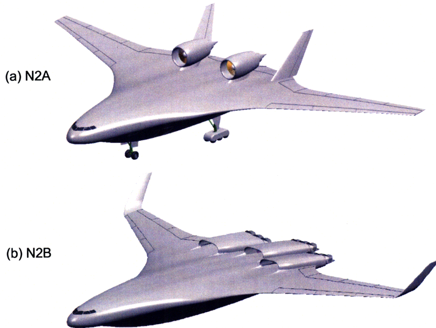
Figure 2-8: Rendering of the SAX-40F based N2A and N2B HWB aircraft [picture courtesy of D. Odle, Boeing]
