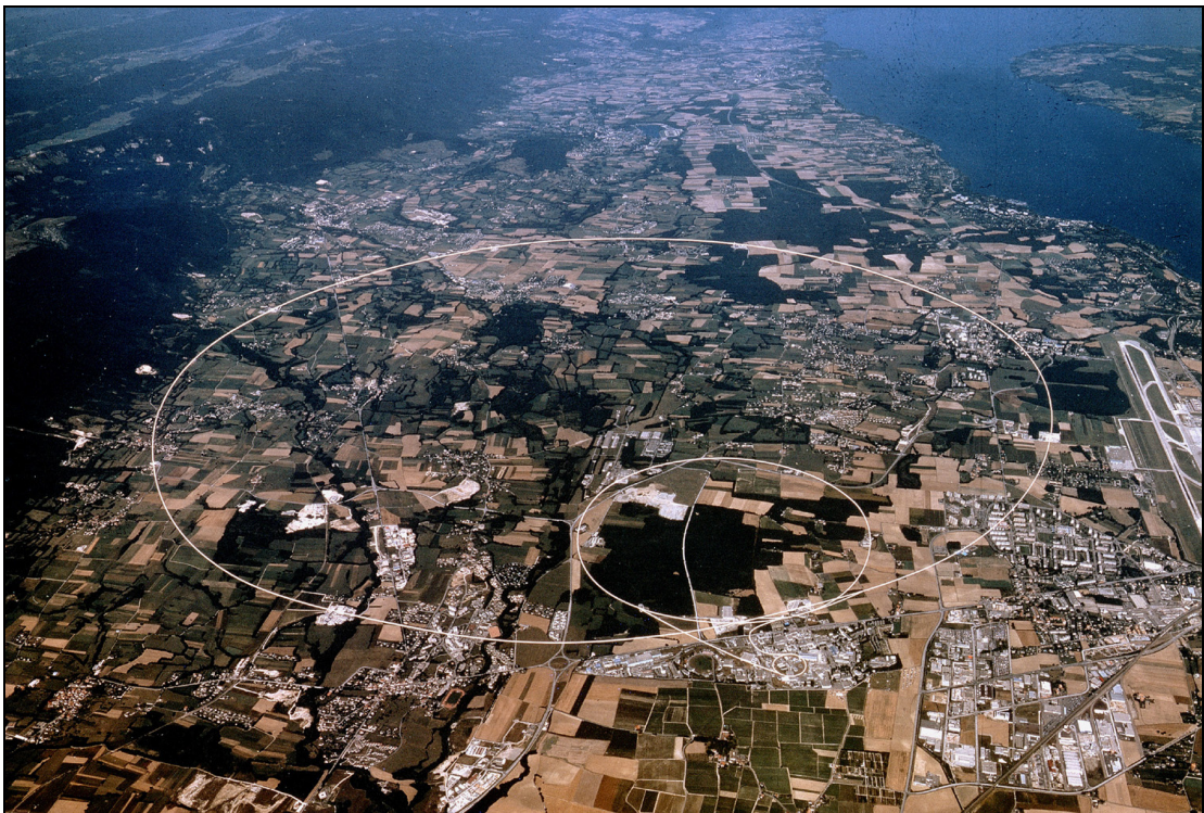
Figure 1.1: Aerial view of CERN and the surrounding region. 3 rings are drawn to show the position of the accelerator complex situated underground. The small ring shows the position of the Proton Synchrotron with a circumference of 600 m, the middle ring is the Super Proton Synchrotron with a circumference of 7 km and the largest ring is the LHC. The Geneva Lake and the Geneva airport can be seen on the right whilst the Jura Mountains can be seen on the left.
