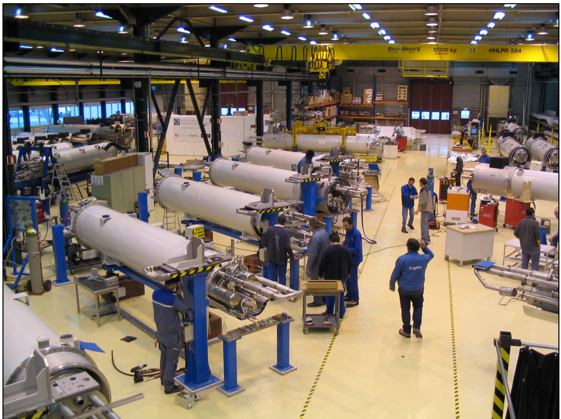
The assembly of the Short Straight Sections.
