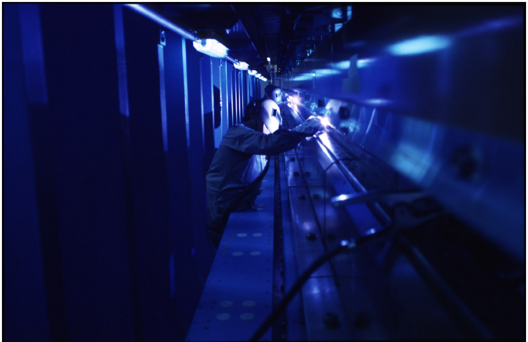
Welding a cryodipole held in place by a hydraulic press.
