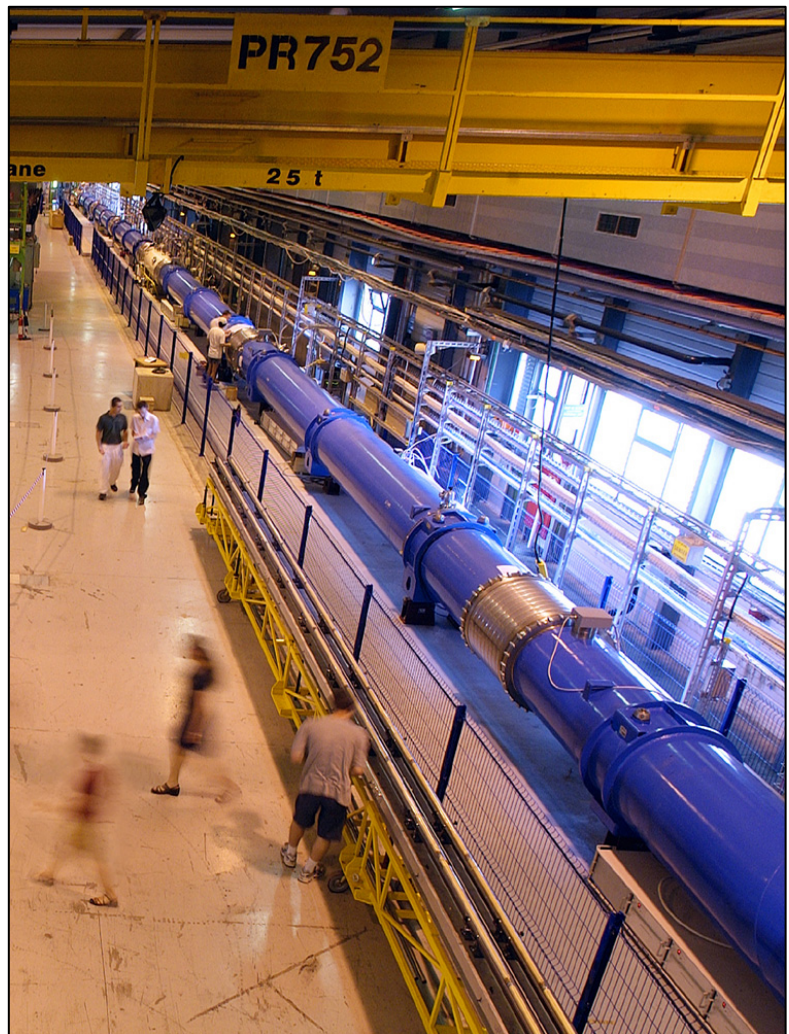
LHC string ready for testing.
