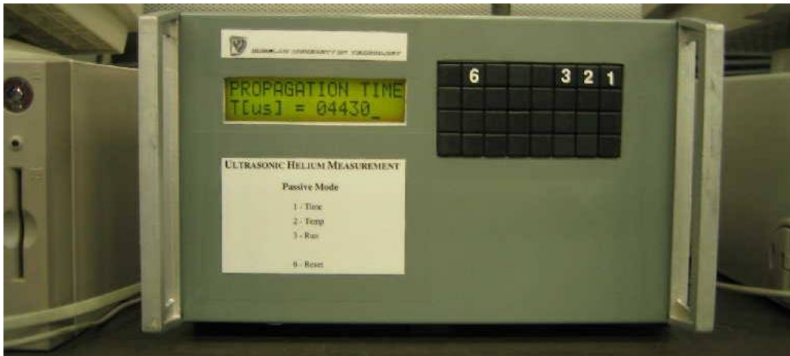
Fig. 6. The control unit placed in the BA80 control room
