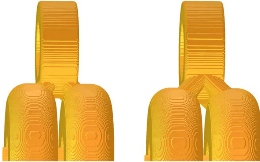
Figure 4: Long coupling slots together with long distances between accelerating and coupling cells (on the right) produce additional edges and therefore an increase of losses.
