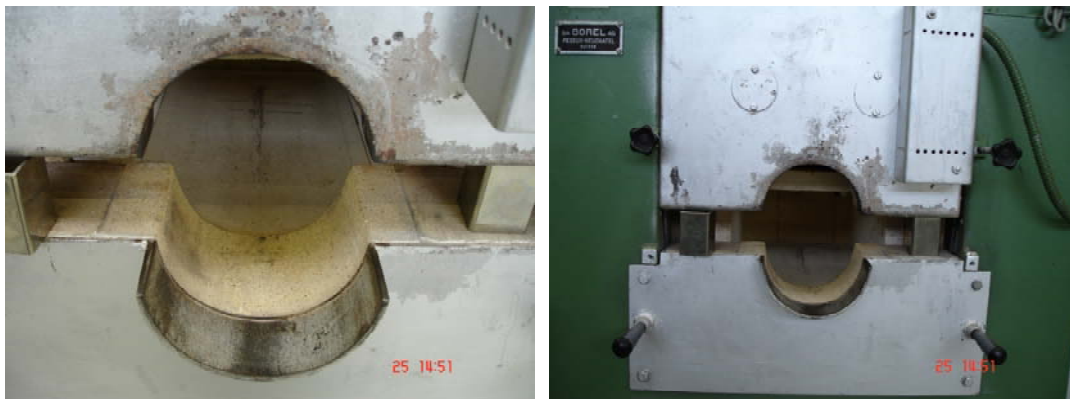
Figure 3. Furnace used to perform the pre-heat treatment.
