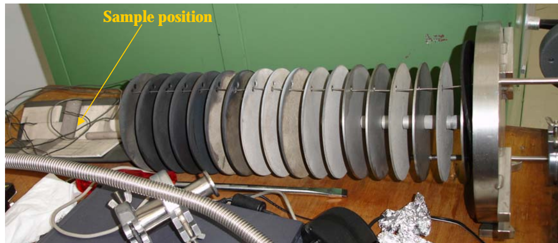
Figure 5. Structure inserted in the furnace to perform the final step of the heat treatment. The sample is put onto some pieces of alumina which act as thermal insulation.
