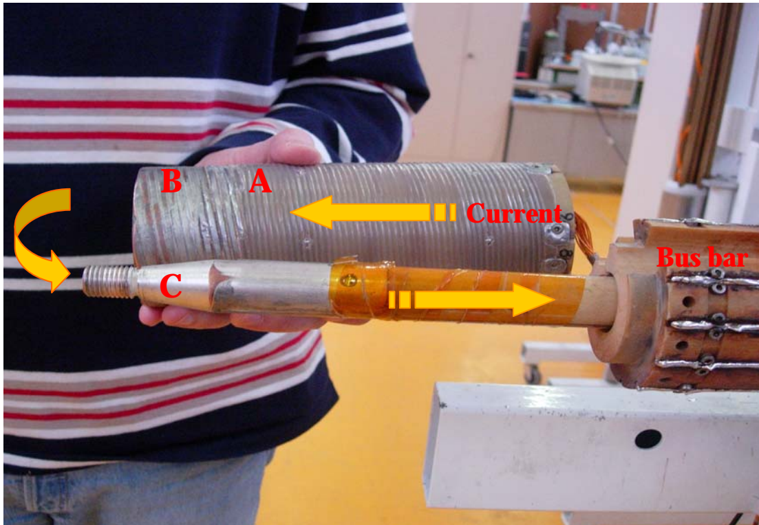
Figure 15. Sample holder for the critical current density measurement of the NbTi strands at CERN.
