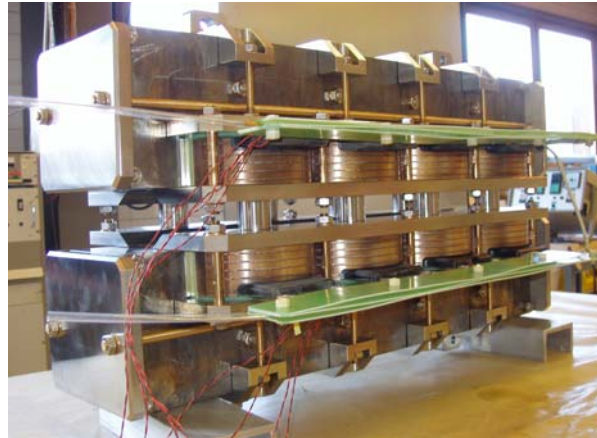
Figure 13. NbTi undulator for the proton beam diagnostics.
