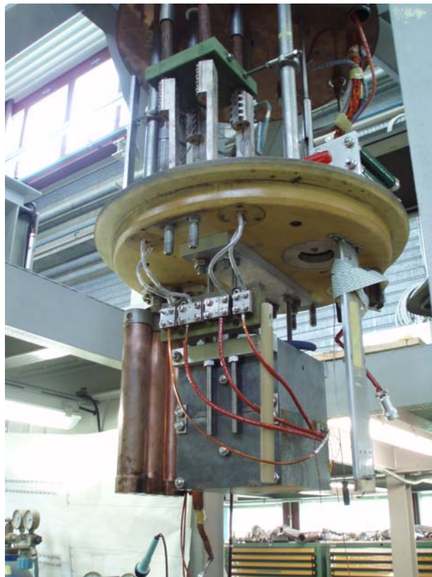
Figure 9. Complete assembly of the magnet as inserted in the cryostat.
