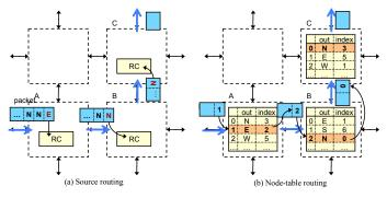
Figure 1: The table-based routing architecture (a) Source routing (b) Node-table routing
