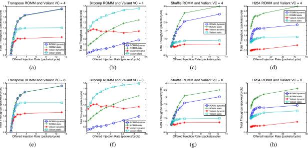
Figure 6: Throughput for ROMM and Valiant under static and dynamic allocation with 4 and 8 VCs.
