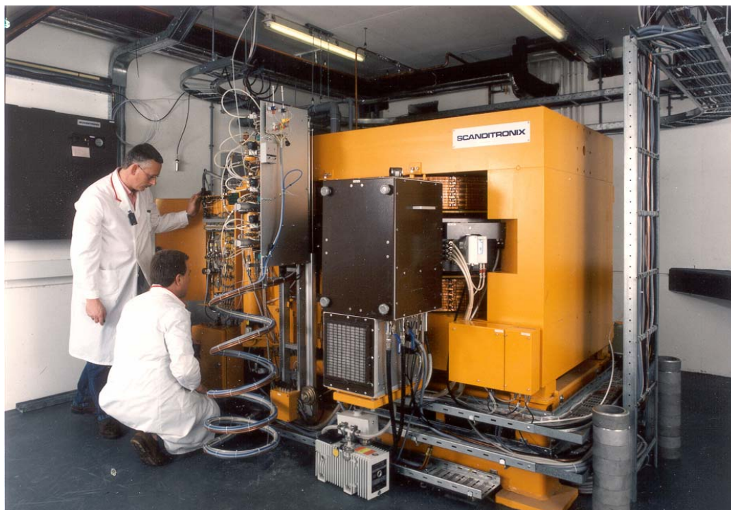
Fig. 1: Scanditronix MC-17F cyclotron as installed in 1991 in the UMCG for the production of ^{11}\text{C} , ^{13}\text{N} , ^{15}\text{O} and ^{18}\text{F} . Beams available are 17 MeV protons or 8.5 MeV deuterons. Targets are mounted at the target ladder at the beam exit of the cyclotron MC-17.
