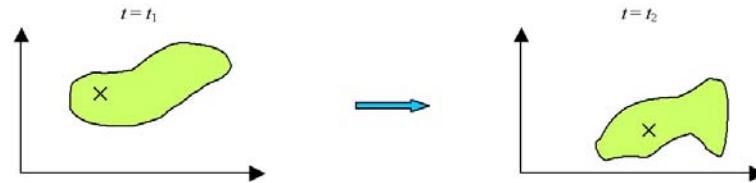
Fig. 1: Liouville's theorem says that the density of points in phase space, measured along the trajectory of a given point (like the one marked by an x) does not change in time
