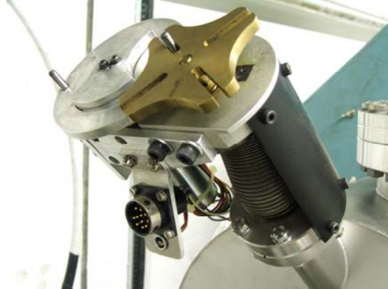
Fig. 21: A rotary mechanism for four screens
