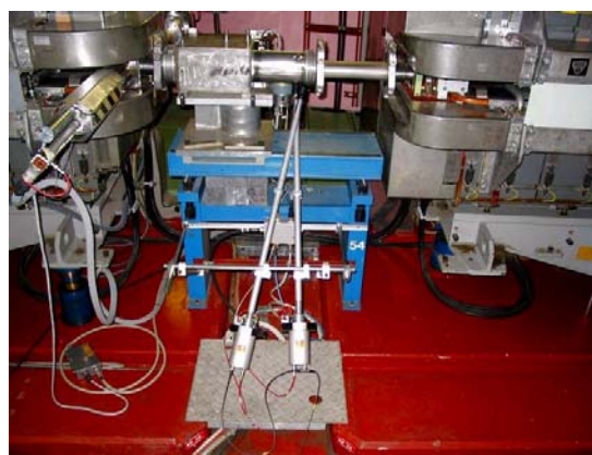
Fig. 24: Fast wire scanner with scintillator and photomultiplier
