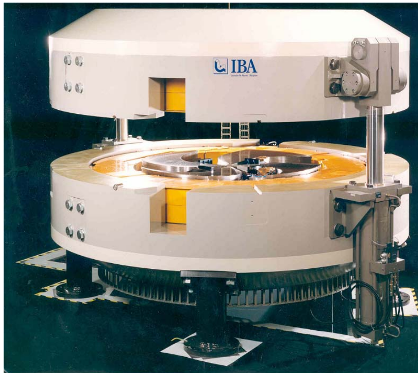
Fig. 6: The IBA C235 is a good example of cyclotrons with the horizontal median plane of the cyclotron magnet
